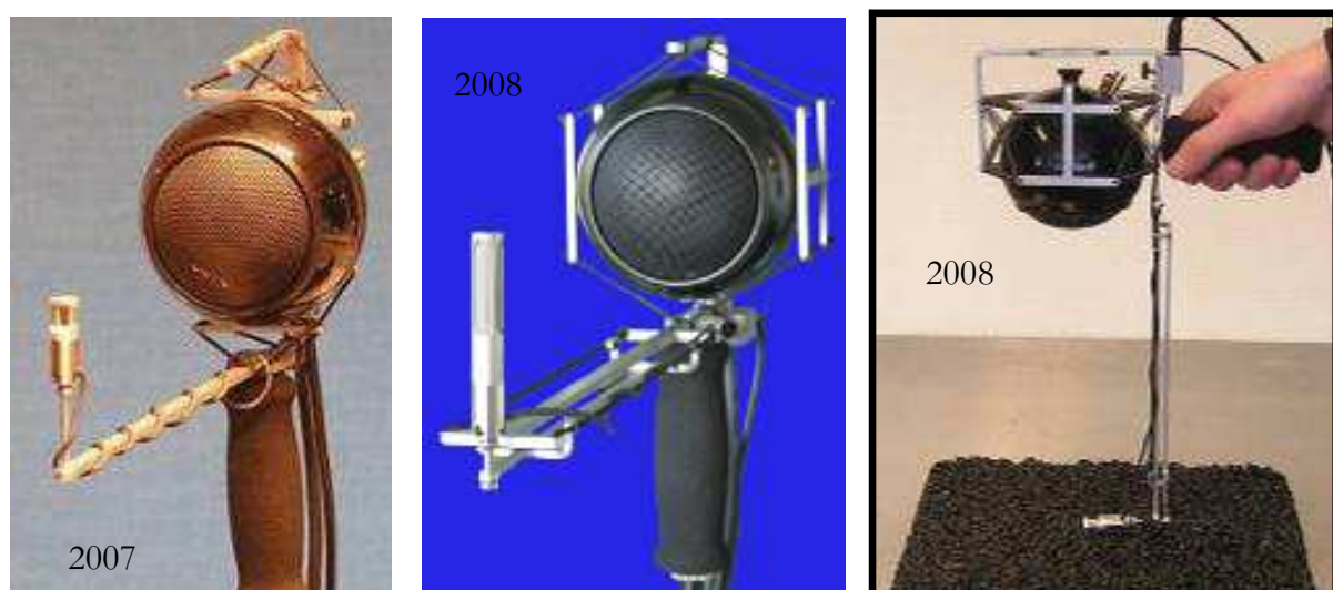
Fig. 4-4. Several versions with a steel grid. Right: The version used up to date.
