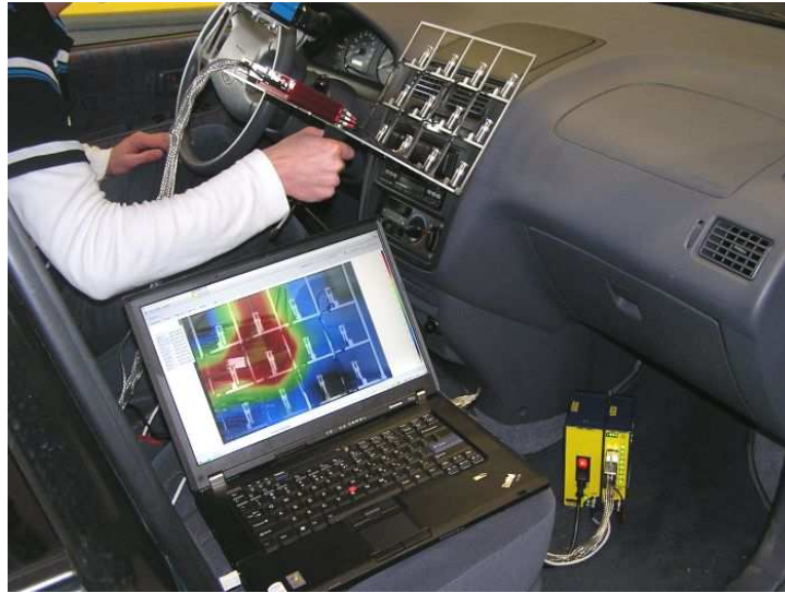
Fig. A-3. Acoustic camera hardware and software.
