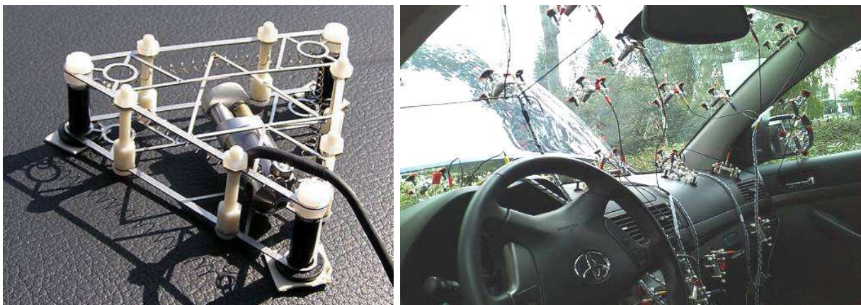
Fig. A-4. Left: probe suspension. Right: Panel noise array mounted in a car.
