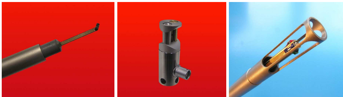
Fig. 2-11. Three main probe types that contain Microflown sensors. Left: scanning probe (1D particle velocity). Middle: PU probe (sound pressure and 1D particle velocity). Right: USP probe (sound pressure and 3D particle velocity).
